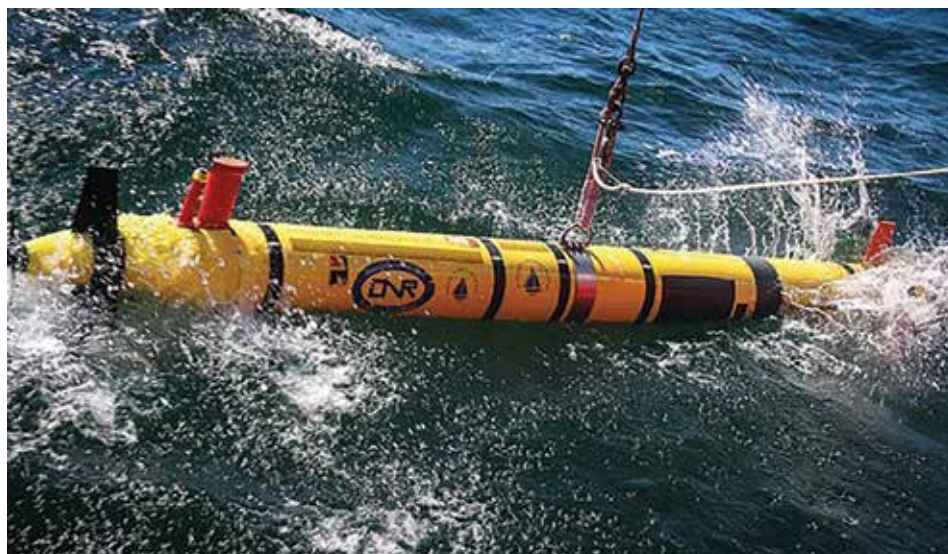
The Office of Naval Research launches a REMUS 600 autonomous underwater vehicle for mine search and identification operations off the coast of Bornholm Island during BALTOPS 2018. The U.S. Navy is among the nations participating in a drone exercise off the coast of Portugal this September. (MCC America Henry/(U.S. Navy)
