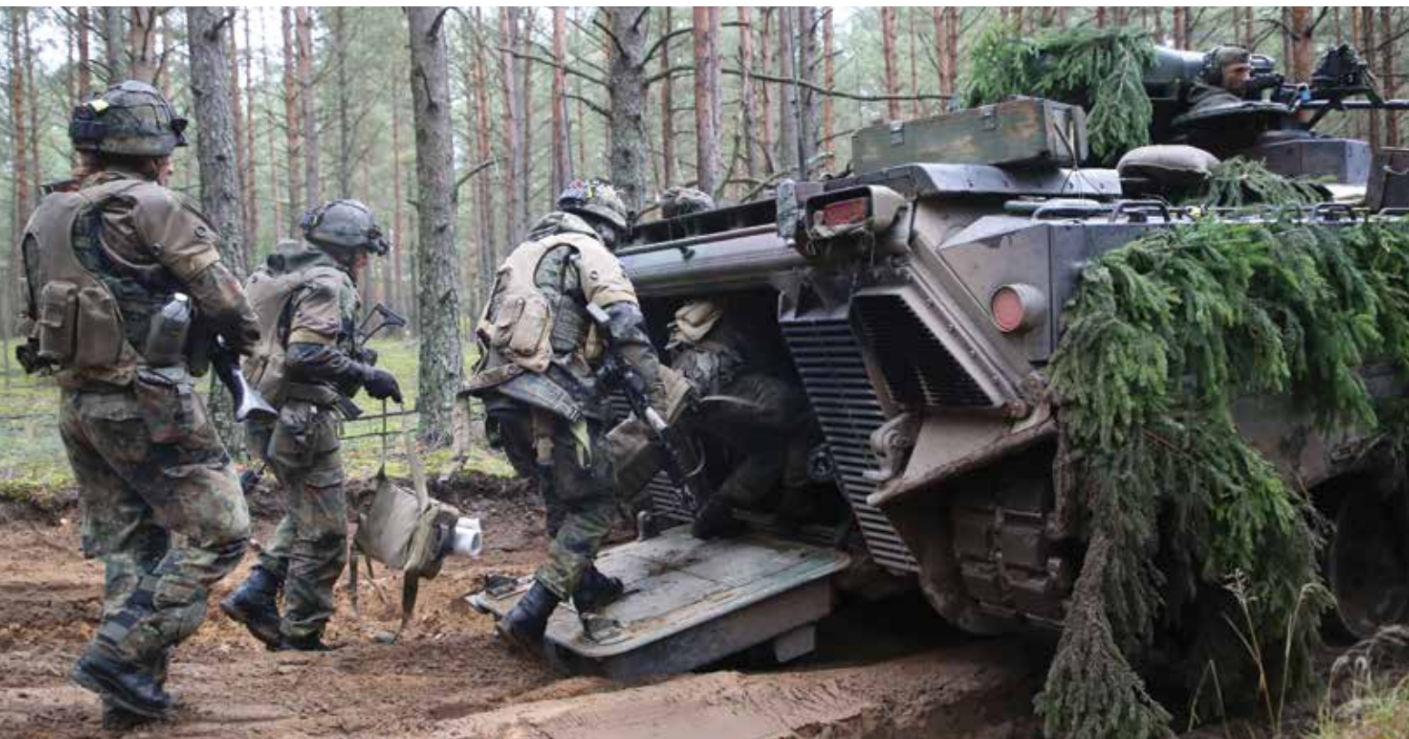
The "Marder" crew consists of 9 panzergrenadiers: Commander, gunner (both in the tower), driver (in the front of the tub) and a troop leader with 5 other grenadiers in the rear combat area.
