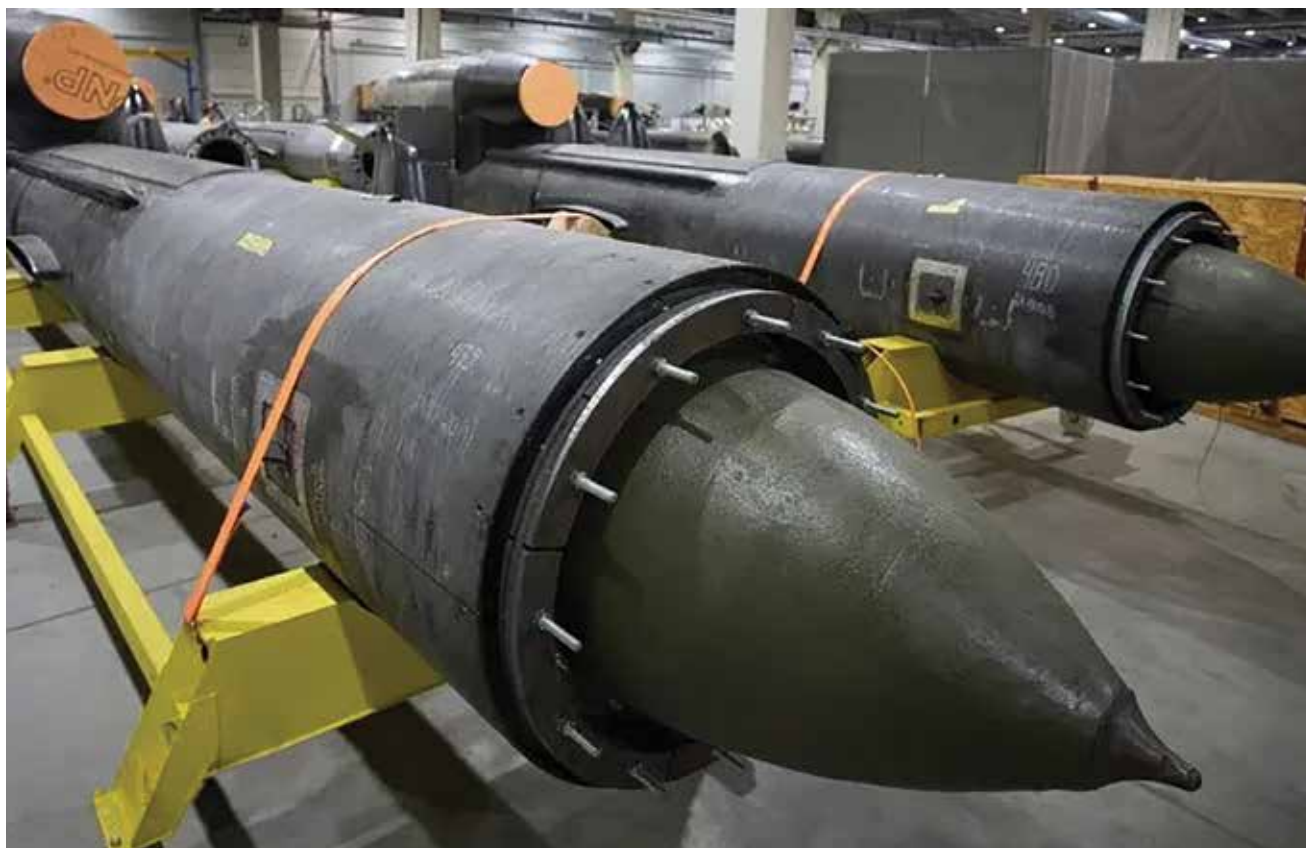
A ton of explosives, the Flamingo's warhead utilized heavy aviation bombs.
