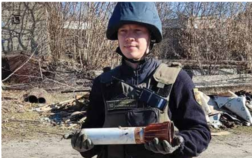
This small object in the soldier's hands is a decoy deployed by Iskander during flight, functioning essentially as a radio-jamming beacon and a heat source.
